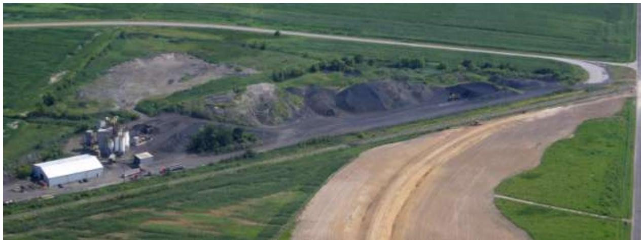
U.S. Minerals uses the bottom ash from Coffeen Power Station for making construction materials. Coal ash is stored in large piles at the industrial site, a half mile north of Coffeen Power Station. The piles of coal ash do not have liners, covers, windbreaks, or silt fences to prevent erosion and release of pollutants to air and water.
