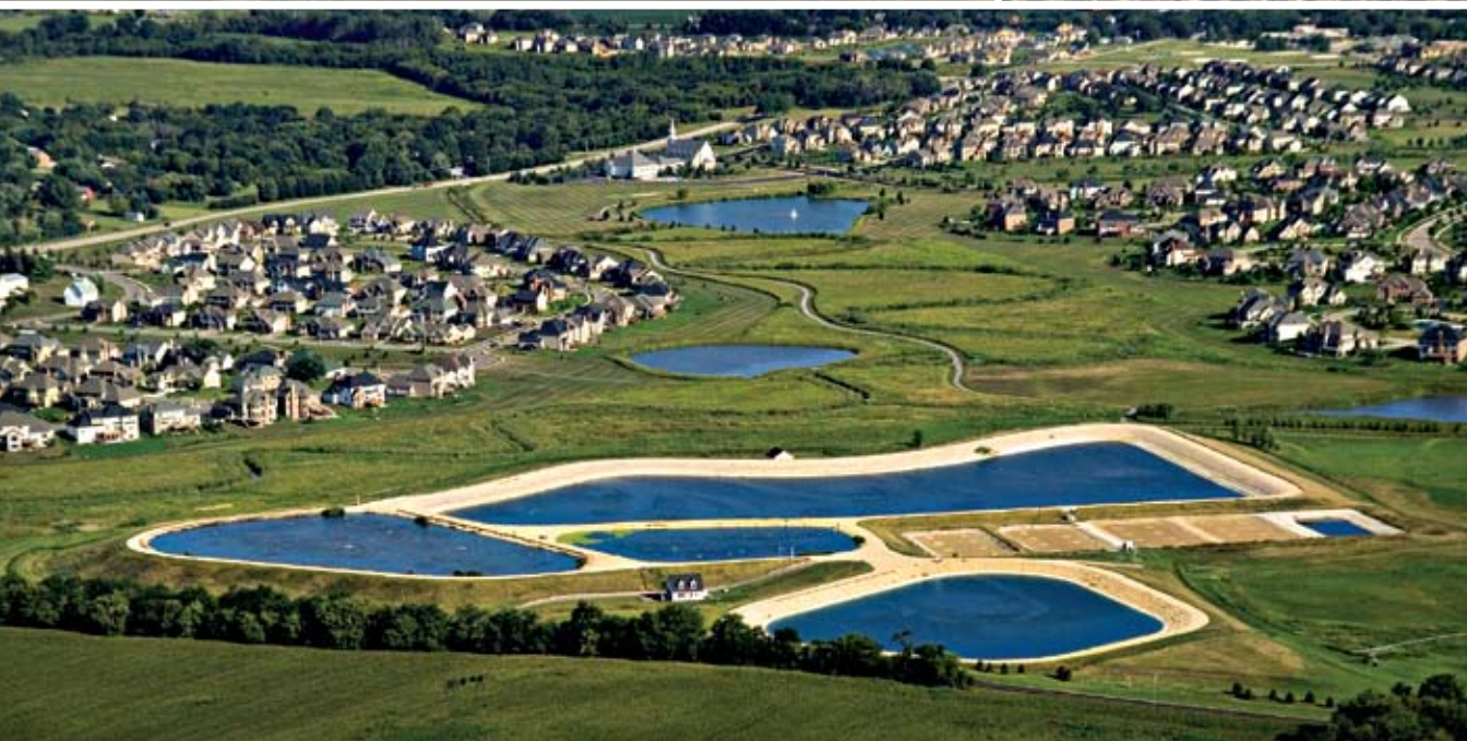
Above From Left: Irrigation of golf course from no-discharge system at Fox Mill, IL, example of agricultural spray irrigation from wastewater treatment plants. Bottom: Fox Mill, a mixed use development community and no-discharge municipal sanitary district in Wasco, Illinois.
