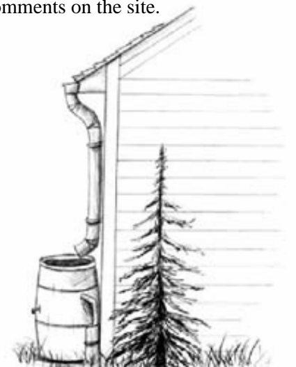
A rain barrel can be used to capture runoff from a roof-top
