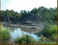
Coal waste is often dumped in wet above-ground pits that can tower up to 80 ft tall and cover over 1 square mile. Mining companies will dispose of hundreds of millions of gallons of harmful coal slurry behind a typical coal slurry dam, which will remain behind permanently after the mines close.
